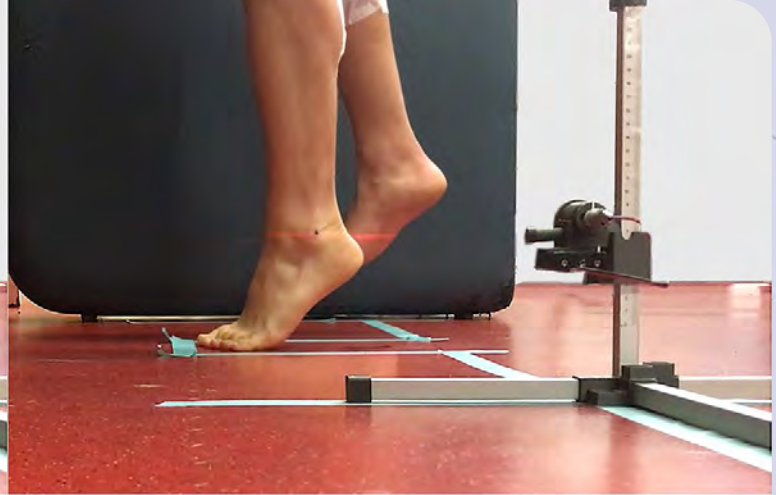
B. Heel rise. The beam of the laser pointer was set at the height of the heel rise.
